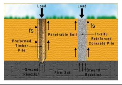
Load is partly taken by shaft, Q<sub>s</sub>, and partly by end, Q<sub>b</sub>
