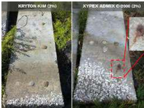
1. Hydrophobic pore blocking 2. Corrosion-inhibiting surface coating
