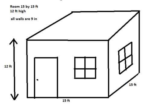
A cutting plane is introduced just above the sill level and upper portion of room above the cutting plane is removed
