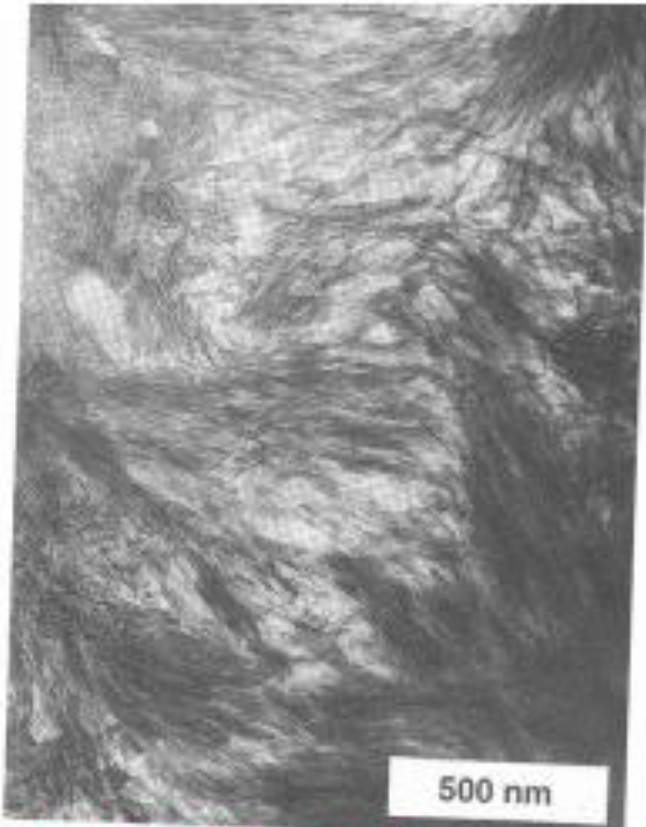
Fine, fibrillar structure, similar to Power's model (typical of \text{Ca/Si} > 1.5 )
