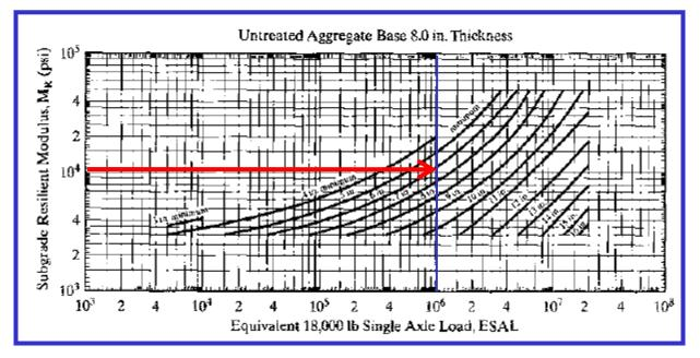
Flexible Pavement Design Asphalt Institute Method-Design Procedure HMA and Emulsified Asphalt Mix Over Untreated Aggregate Base Design charts for pavements consisting of a HMA surface, an emulsified asphalt base and an untreated base are currently not available.
