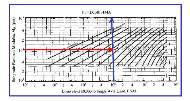
Figures are the design charts for types I, II and III emulsified asphalt mixes respectively. The chart gives the combined thickness of HMA surface course and emulsified asphalt base course.
