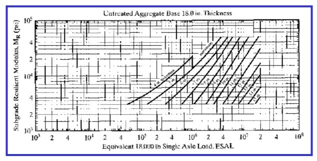
**Exible Pavement Design Asphalt Institute Method-Design Procedure HMA over Untreated aggregate base-Numerical problem** Given  $M_R$ = 10,000 psi and ESAL= 10<sup>6</sup> and an untreated aggregate base 8 in. thick, determine the thickness of the HMA required.
