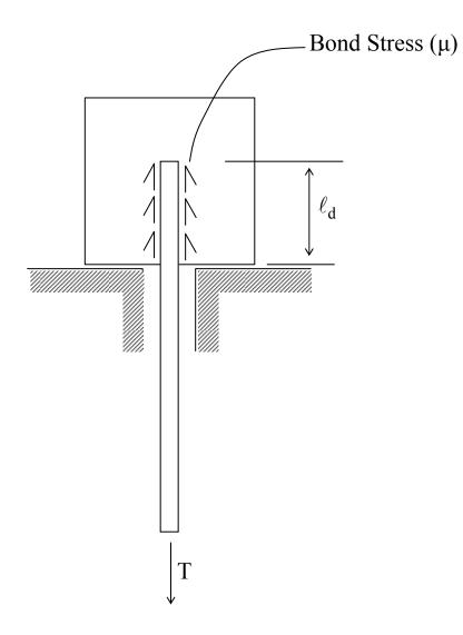
Fig. 11.1.Experimental Setup For Pullout Test.
