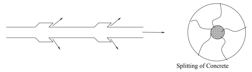
Fig. 11.2. Cracking in Concrete Due to Pull in Steel Bar.
