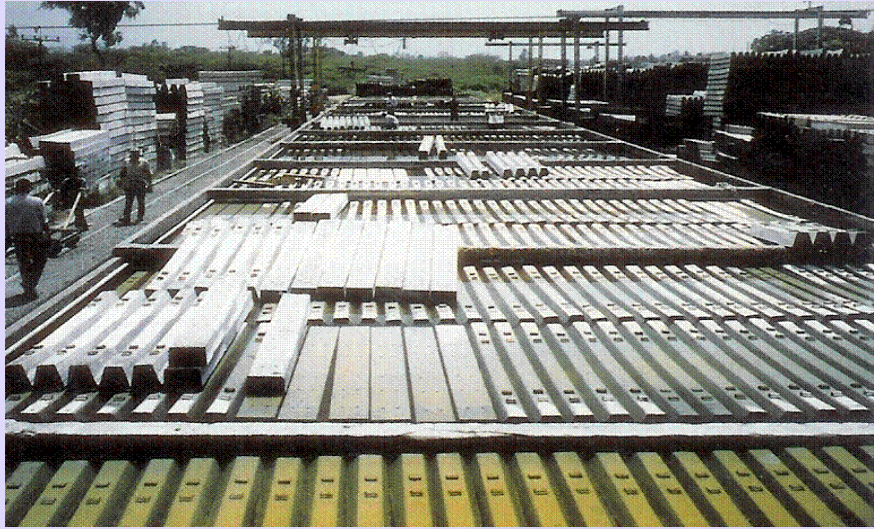
Figure 1-2.6 Linearly prestressed railway sleepers
