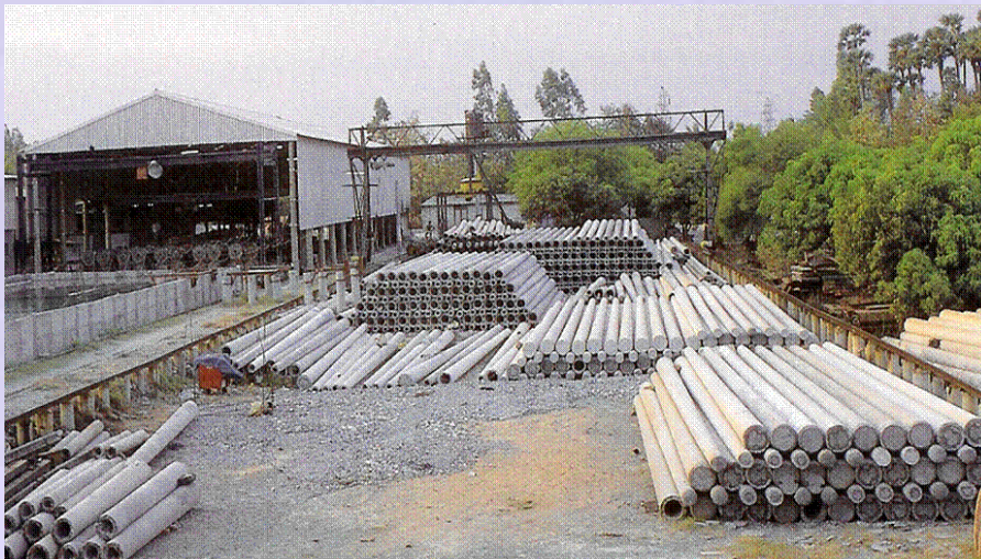
Figure 1-2.4 Pre-tensioned electric poles
