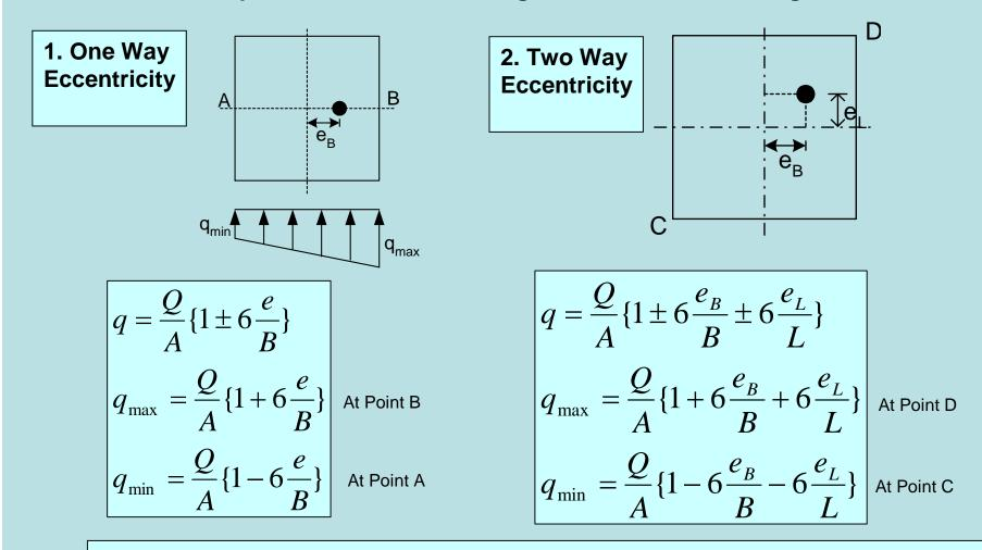
$e_B$  or  $e_L$  should be less than B/6 or L/6, respectively, to avoid negation pressure under the footing in case of one/two way eccentricity.
